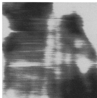
Figure 17: Stacked radial lamellae of \alpha -m spherulite, T_c=125^\circ\text{C} , AFM scan, 250\ \text{nm} \times 250\ \text{nm} , NanoTip
