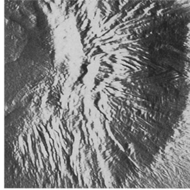
Figure 9: \alpha -II spherulite, AFM scan, force mode, 15\ \mu\text{m} \times 15\ \mu\text{m} , Ultralever
